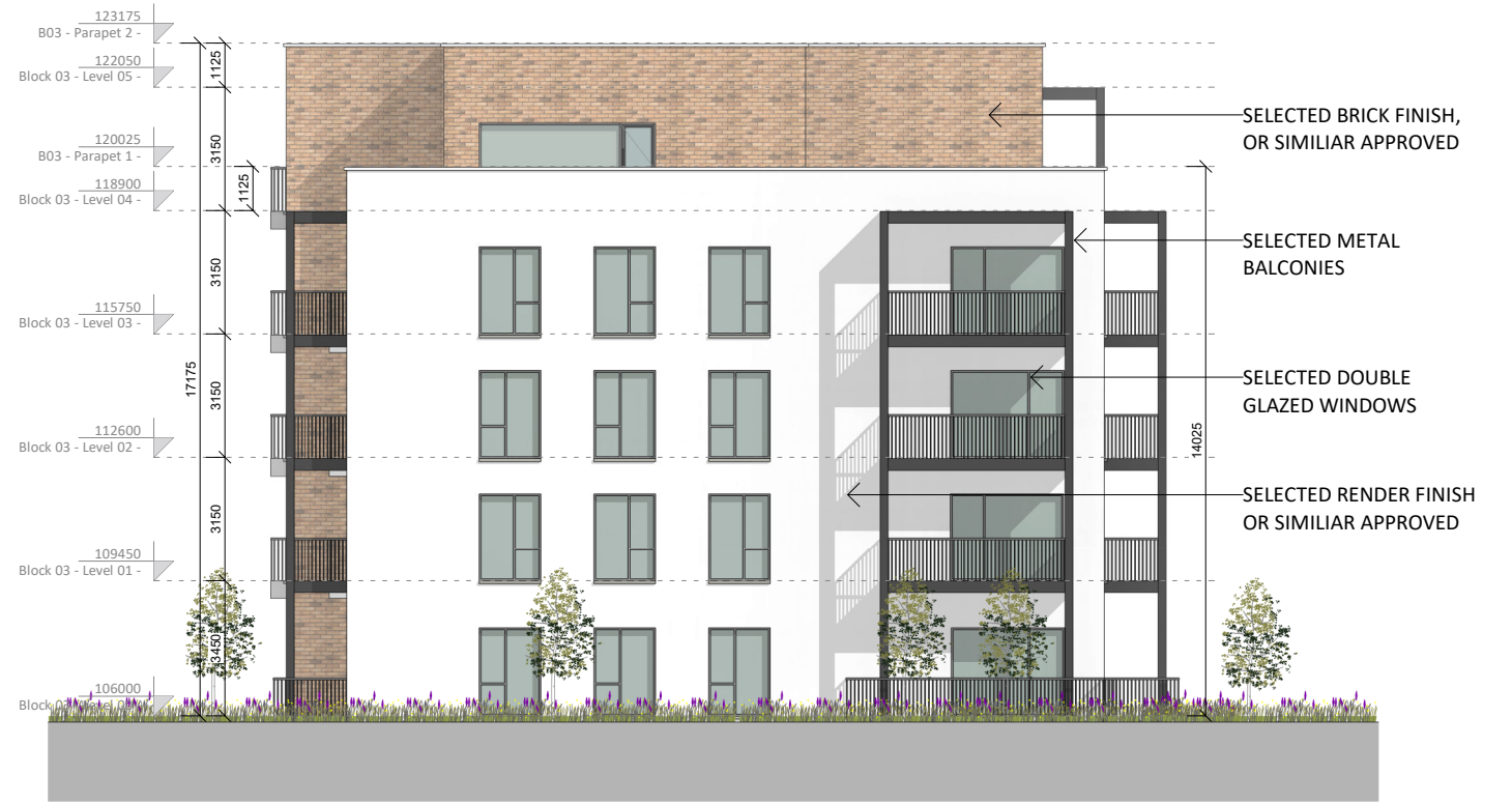
② Block 03 - South Elevation 1 : 200
